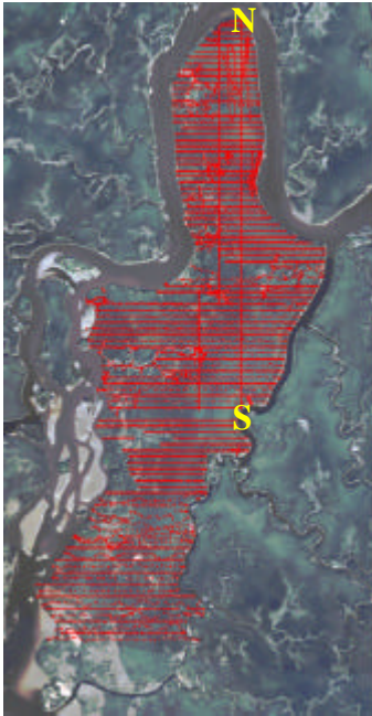
Figure Y. Post map showing position and track of RTK GPS topographic survey. Each dot represents a single x,y,z coordinate for the marsh surface. S-N elevation transect location indicated on post map.
